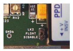
Figure 2-1. Float Enable/Disable Jumper
